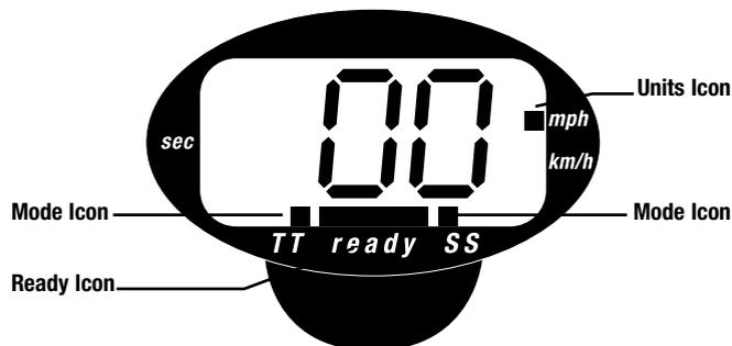
Once a swing is experienced, the Display will toggle (alternate) from Tempo Time to Swing Speed, as previously illustrated in Figures 6 and Figures 4 or 5, depending on the units chosen. However, the TT Mode Icon is the Decimal Point in the TT Mode, and the SS Mode Icon does not appear when toggling into the SS Mode.
