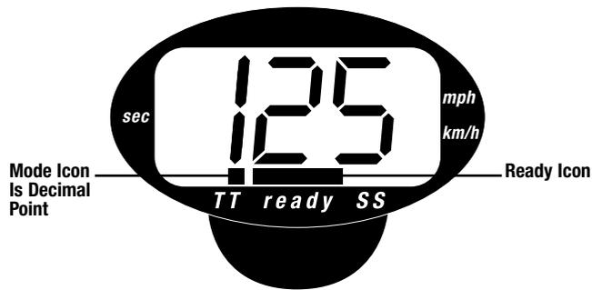
The SSRTT measures the time from the clubhead takeaway start of the backswing to the return of the clubhead at ball impact. The TT measurement is displayed in seconds, from 0.50 seconds up to 4.00 seconds maximum, with tenths and hundredths of a second shown by the 3-digit Display. The Mode Icon represents the decimal point when in the TT mode. Figure 6 illustrates a Tempo Time of 1.25 seconds
